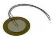
A transducer plays a very important role in any instrumentation system. An electrical transducer is a device which can convert the physical quantity into a proportional electrical quantity such as voltage or electric current. It converts any quantity to be measured into usable electrical signal. This physical quantity, which is to be measured can be pressure, level, temperature, displacement etc. The output which is obtained from the transducer is in the electrical form and is
