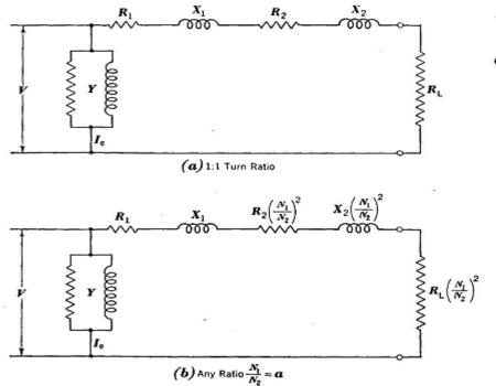
15. Draw the equivalent circuit of a transformer referred to primary. (Remembering)
