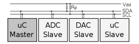
One master (a <u>microcontroller</u>), three slave nodes (an <u>ADC</u>, a <u>DAC</u>, and a microcontroller), and <u>pull-up resistors</u>  $R_{p}$ .
